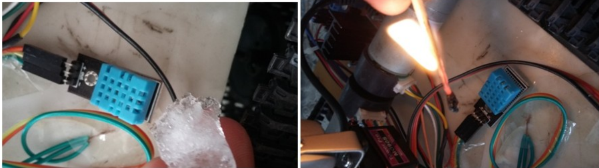
Figure 10: DHT-11 sensor testing in presence of ice and fire
